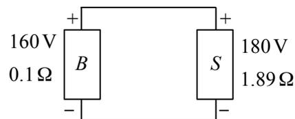
The total length of the connecting wires is 4 m. Calculate the cross-sectional area of the connecting wires made of copper if the constant charging current is 10 A. (Resistivity of copper is  $1.72 \times 10^{-8} \Omega \text{ m}$ )
