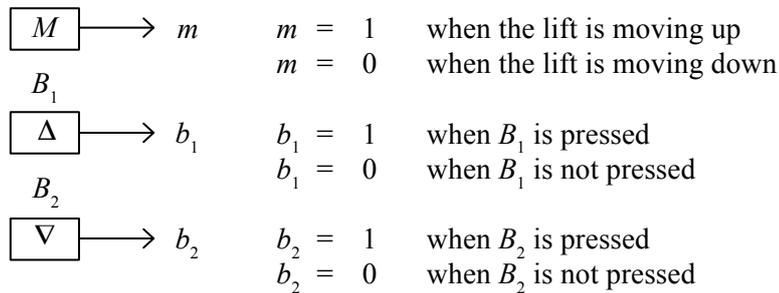
A logic circuit has to be designed to meet the following conditions.
